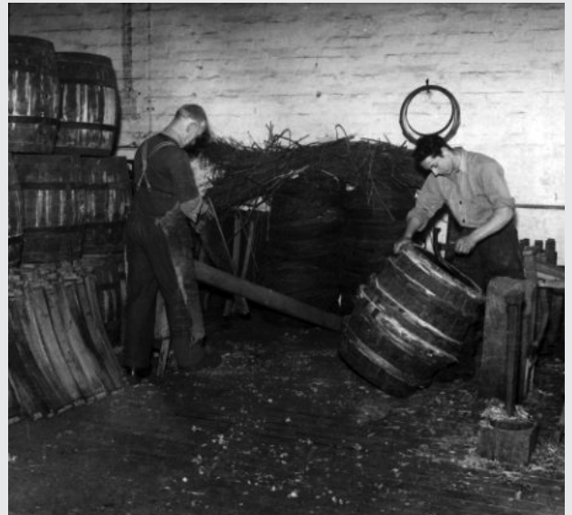
A Cooper and his apprentice at work making barrels in Factory Cooperage
